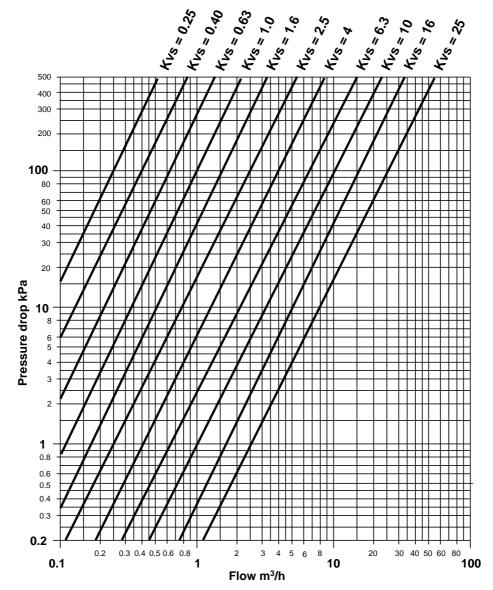
Kvs = Flow coefficient : Flow in  $m^3/h$  with open valve and pressure drop of 100 kPa. 100 kPa = 10 mWG = 1 bar
