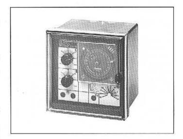
To adjust the desired room temperature Ta, parallel shifts of the selected heating curve can be made by means of the potentiometers "Sun" (fig. 2.4) and "Moon" (fig. 2.5). In this way it is possible to establish two different values for Ta: a "Normal" value for periods of occupation and a "Setback" value for unoccupied periods.
