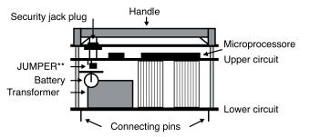
\*\*Without jumper : Data can be changed only with security jack plug With jumper : Data can be changed even without security jack plug
