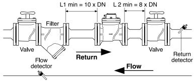
L1 and L2 min. according to UNI EN 1434-6 Regulations
