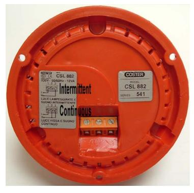
By wiring Live to terminal 1 and Neutral to terminal 3 you get an intermittent audio tone. By linking Neutral across to terminal 2 you get a continuous tone.
