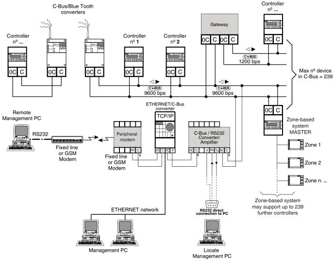
The example shows the C-Bus connections and all the available modes in which the systems may be managed remotely, even simultaneously:
