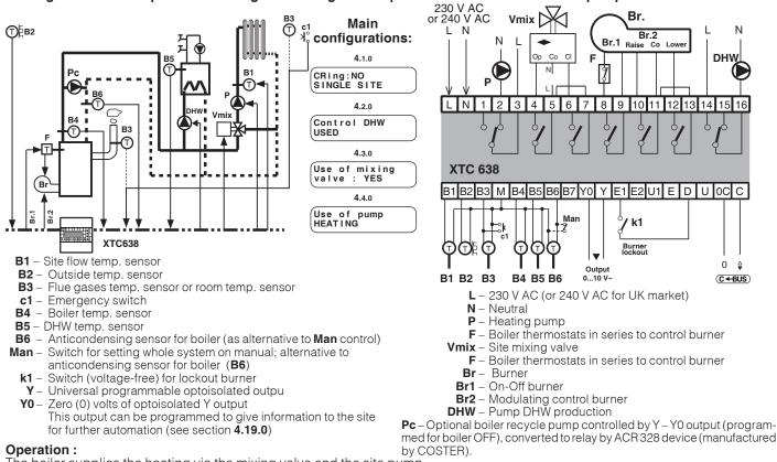
The boiler supplies the heating via the mixing valve and the site pump. The **DHW** pump is switched on when the DHW calorifier calls for heat.
