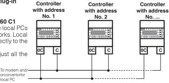
XTC 638 can communicate at various speeds (see page 27, display 4.26.0). If on the site were to be connected in C-Bus other devices having different speeds, it would be necessary to bring into line the speeds of all the units and of the modem.
