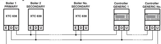
The XTC 638 controller of the primary boiler controls, via C-Ring, all the secondary boilers in order to achieve the sequence, whilst, still via C-Ring, it communicates with the other COSTER controllers in order to have all the information regarding the user outlets. On the basis of this information it decides on the best strategy for the system.
